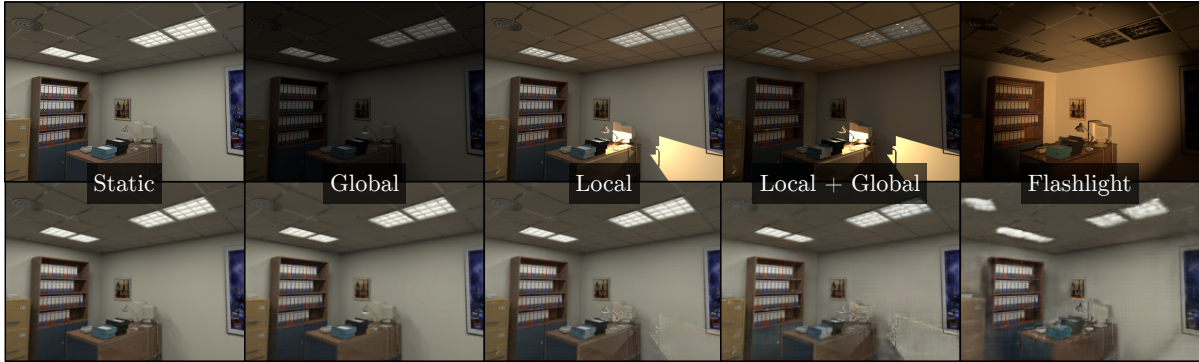
Figure 4.3: Top row : Sample images from the ETHL/syn1 sequences captured at the same pose under different illumination conditions. Bottom row : The same images with a learned transformation that attempts to re-illuminate each image under the “Static” condition.
