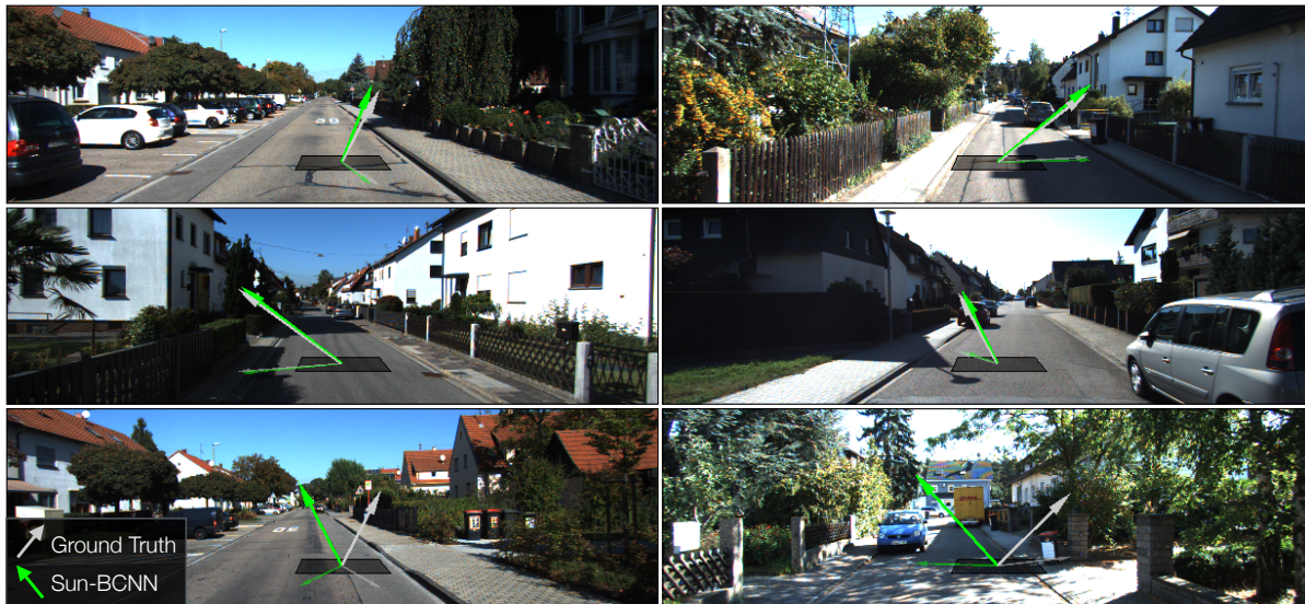
Figure 3.12: Visualization of Sun-BCNN predictions and associated ground truth sun directions on KITTI sequence 05. Top two rows : Sun-BCNN produces accurate predictions in a variety of azimuth values. Bottom row : Poor results occur rarely due to shadow ambiguities.
