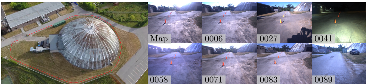
Figure 5.6: Aerial view and corresponding sample frames from multiple traverses of the 250 m path from the UTIAS In The Dark dataset (Paton et al., 2016), which exhibits substantial variation in illumination conditions over a full day-night cycle.
